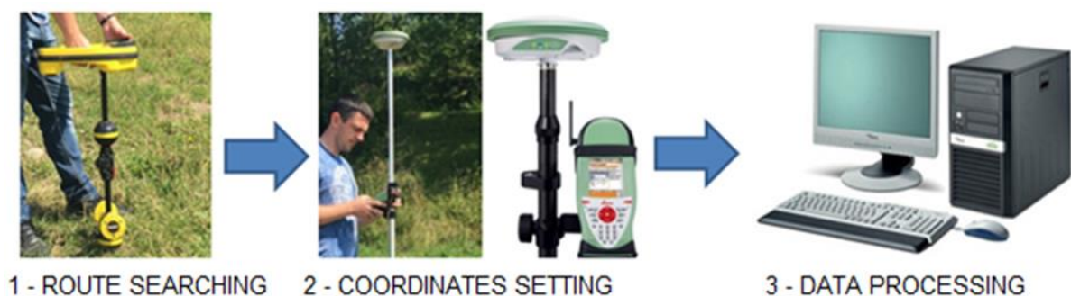
Fig. 3. Procedure for obtaining pipeline SSS data
